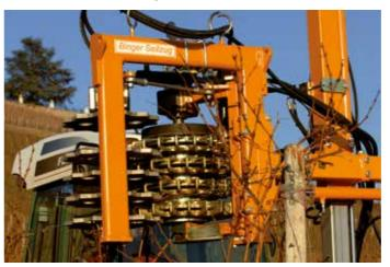
The speed of rotation of the pressure discs and screen is adjustable so that pruning can be adapted to the running speed.
