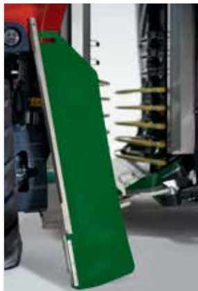
The lightweight row wipers (left) can be easily and quickly removed and reinstalled for maintenance and cleaning.
