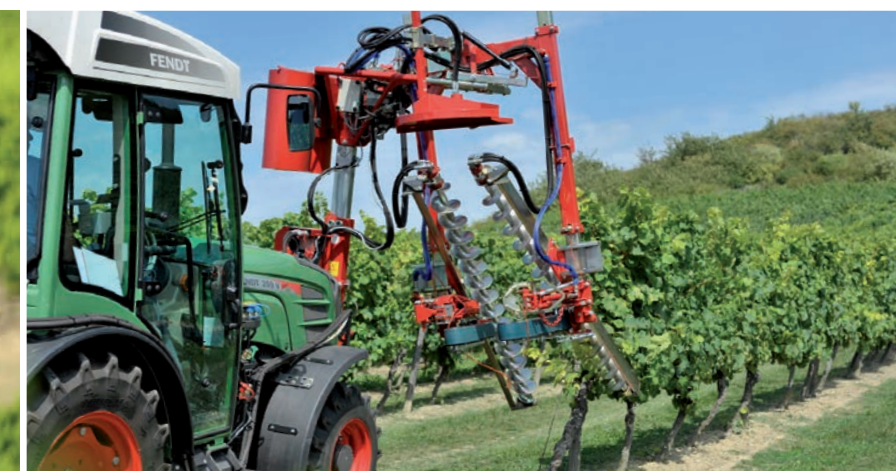
Shoot Binder with belt guides and hydraulic top cutter
