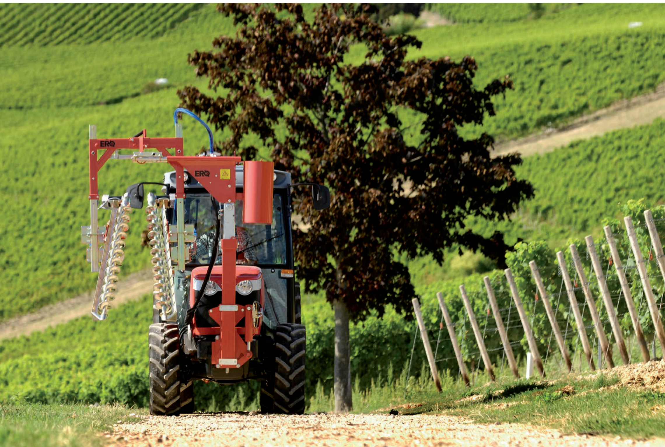
Shoot Binder with belt guides and hydraulic top cutter
